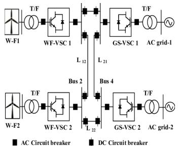
Fig. 1: Four-terminal voltage source converter dc transmission
